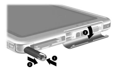
Removing the Pen and Opening the Connector Cover
